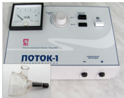
Fig. 1. The control unit of the iontophoresis device and the bath-tube cathode (bottom left).
