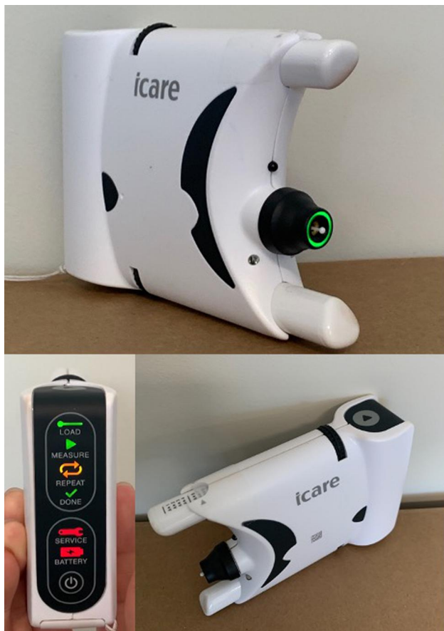
Figure 1 Icare HOME tonometer with a green light (top panel) that reassures that the device is held properly.
