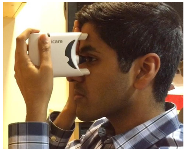
Figure 2 Icare HOME correctly positioned at 90° to the patient’s face.
